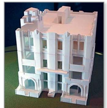
its current modeling. 3D Reprographics built walls as thin as 0.04 in. and found that a 0.08-in. wall gave them the strength and features they required.
